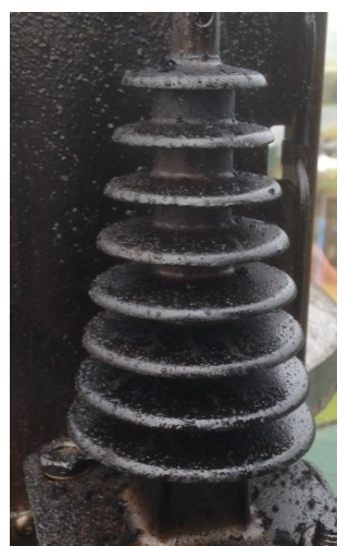
Insulator on coal-wood fire, monitoring round, 27 June
