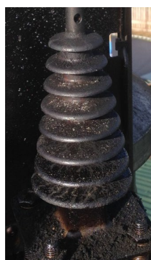
Insulator on coal-wood fire, third monitoring round, 28 July
