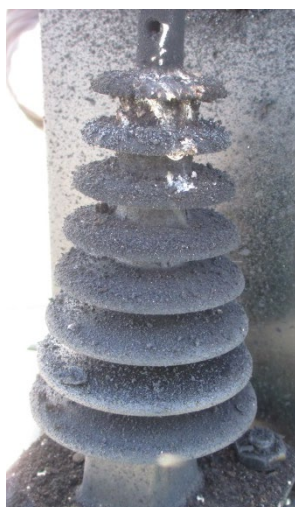
Insulator on coal fire, third monitoring round, 28 July. Note damage on top
